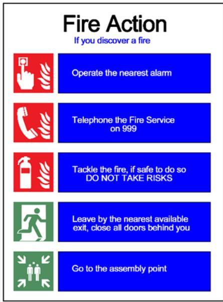
The content of an action plate depends upon the building use and features. For example in a hotel where there is no lift, it is pointless in advising the reader not to use the lift.
